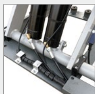
Double acting hydraulic system.
